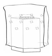
**Step2.** Place the log back into the product box. Place the humidity tent over the box by pulling the open end of the tent down as indicated in the right figure.
